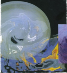
The vortex-induced suction energy draws even the finest of oil films towards the centre.
