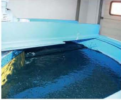
1 st stage: scraper wiper takes away the sludge
